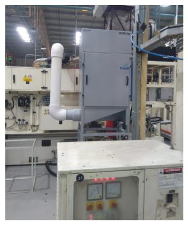
Individual filter APL-DPS- 1100 has been designed for small and medium sized machine tools. The compact design uses very little space. The filter can be flexibly installed on or beside a machine. Energy efficient and powerful, it filters out particles of up to 0.1 µm from air volumes of up to 1000 m³/h. The optimum solution for oil smoke as well as oil and emulsion mist filtering.
